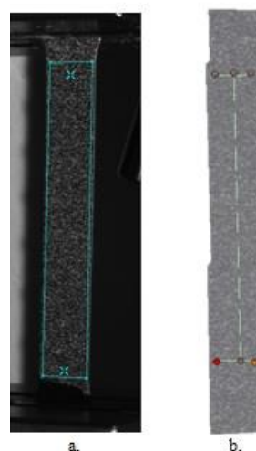
Figure 4. (a) Correlation area with two starting points, (b) Virtual line gauges.
