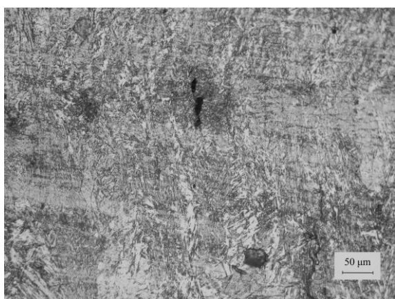
Figure 11. Microstructure of weld nugget-Sample I-200 x magnifications
